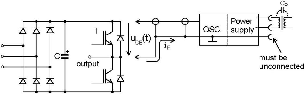
**Fig. 2:** Example of power electronics measurement
