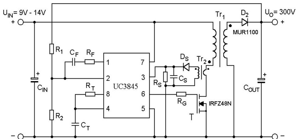
**Fig. 4:** *Wiring diagram of a converter*
