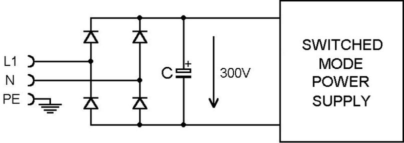
**Fig. 3:** Input side of an oscilloscope
