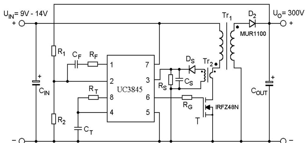
**Fig. 4:** *Wiring diagram of a converter*
