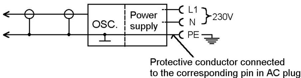
**Fig. 1:** *Oscilloscope connection to the mains*
