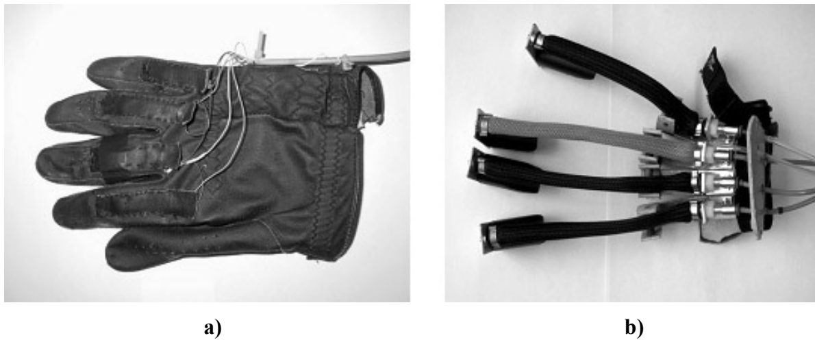
Fig. 2: The position-sensing glove (a) and the exoskeleton structure (b).
