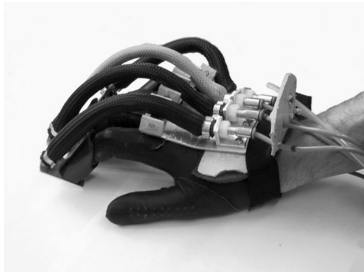
Fig. 1: Haptic Glove with Pneumatic Muscles.
