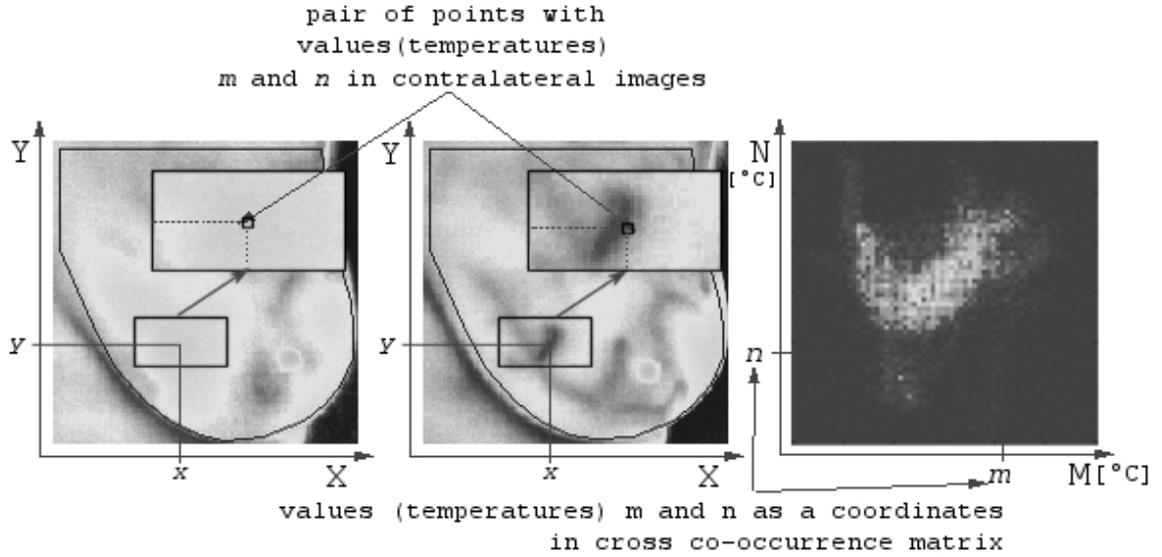
Figure 4: Illustration of acquisition of cross co-occurrence matrix
