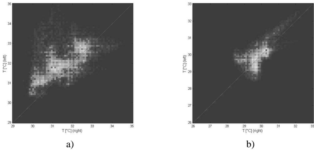
Figure 5: Example of cross co-occurrence matrices for thermogram from fig.1; a) positive thermogram; b) negative thermogram
