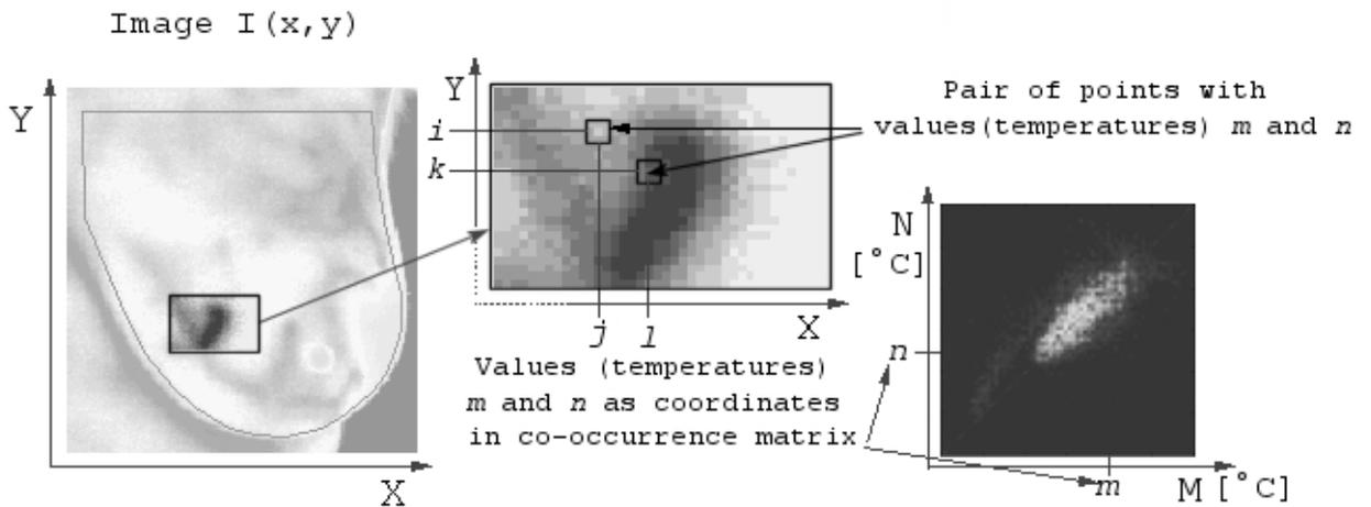
Figure 2: Illustration of acquirement of spatial co-occurrence matrix
