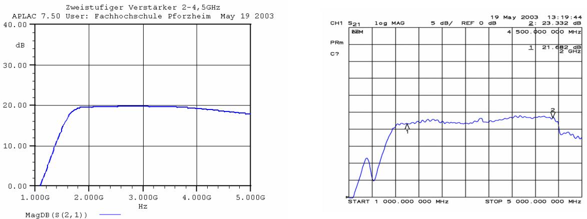
**Fig. 3:** Simulation (left) and measurement (right) of  $S_{21}$
