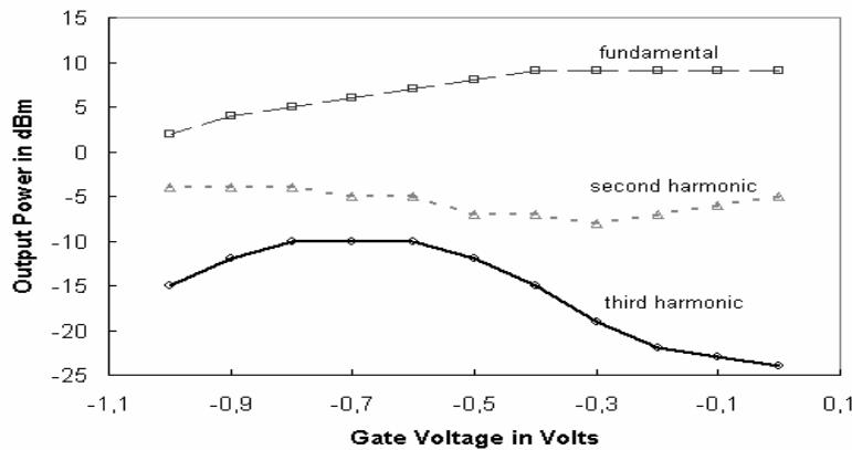
**Fig. 4:** Power of harmonics over gate bias voltage  $U_G$  (MGF1302, +7 dBm in)
