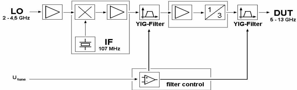
**Fig. 1:** Block diagram of the tracking generator
