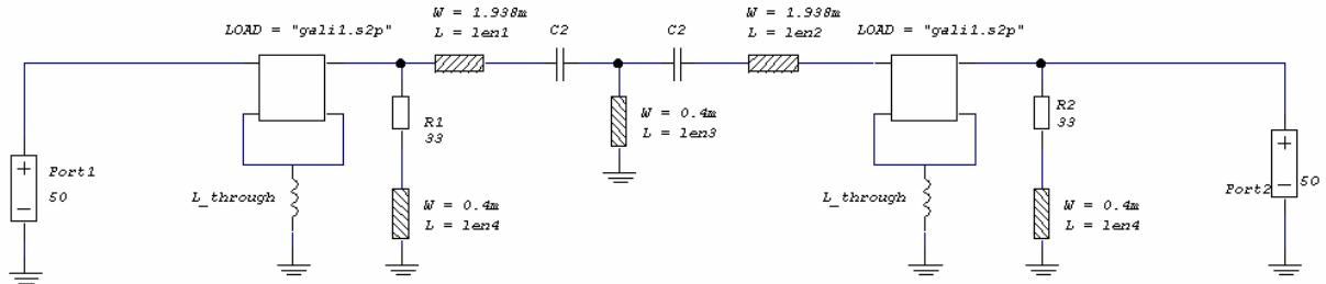
**Fig. 2:** APLAC simulation circuit of two-stage amplifier
